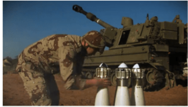
Above: Israeli Top Gun course correction fuses on 155 mm shells
