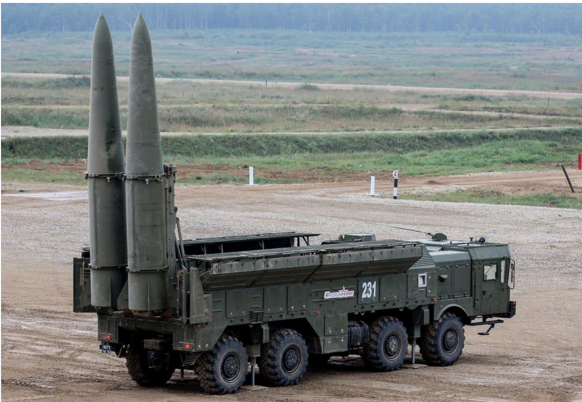
Iskander missile on Transporter Erector Launcher
