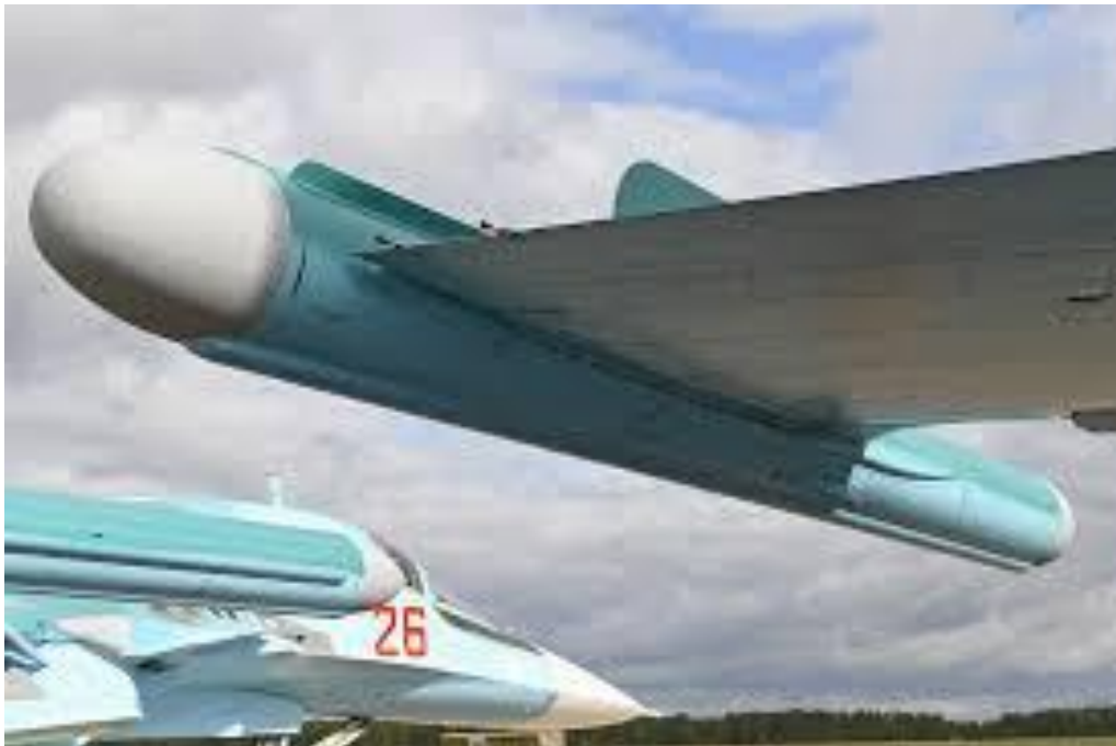
Khibiny EW pods installed on the wings of two Flankers
